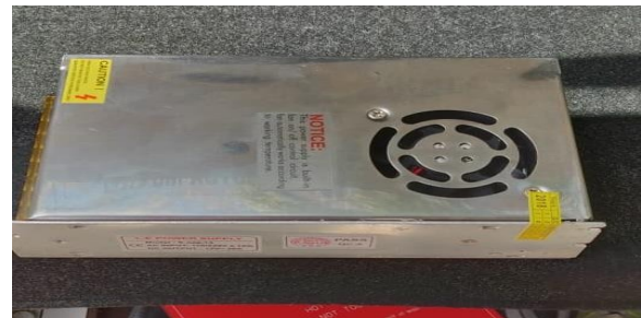
Figure 8: Power Supply for 3D Printer
